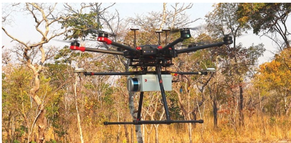
Chart 20: Rousescene LiDARPod mounted on a DJI M600 Pro, Angola
