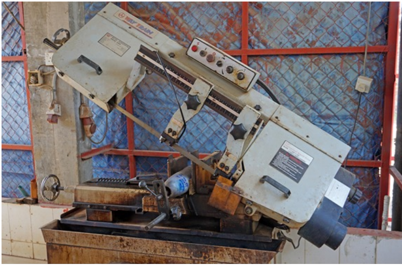
Chart 29: Remotely operated bandsaw for munition cutting 50
