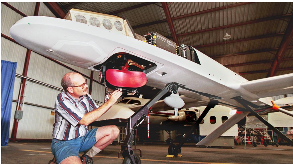
Chart 21: Lynx SAR mounted on a General Atomics I-Gnat UAV
