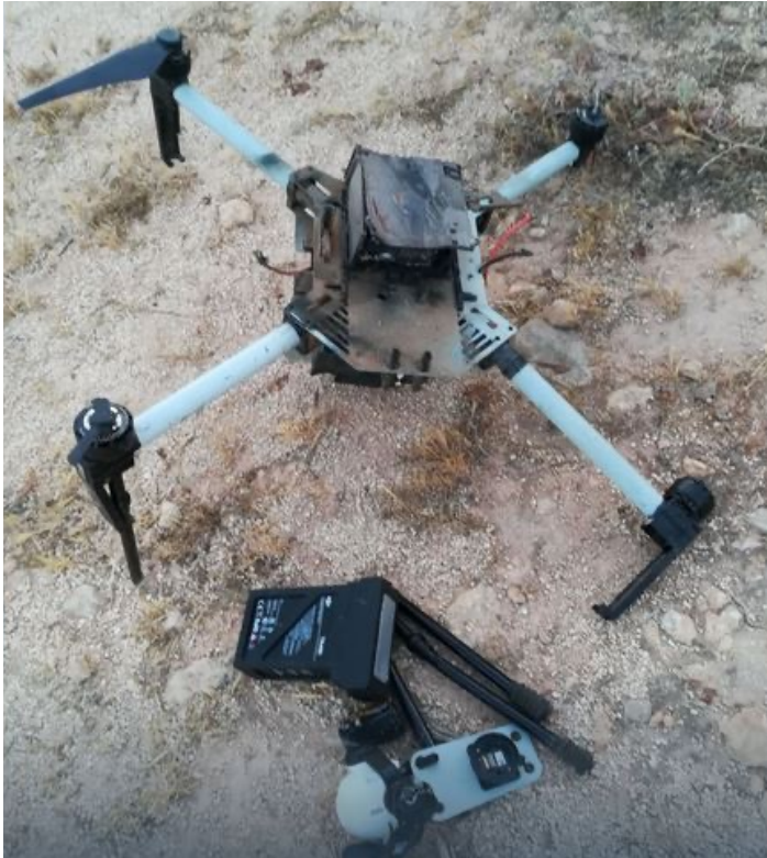
Chart 25: Small UAV adapted to deliver IEDs recovered, Libya
