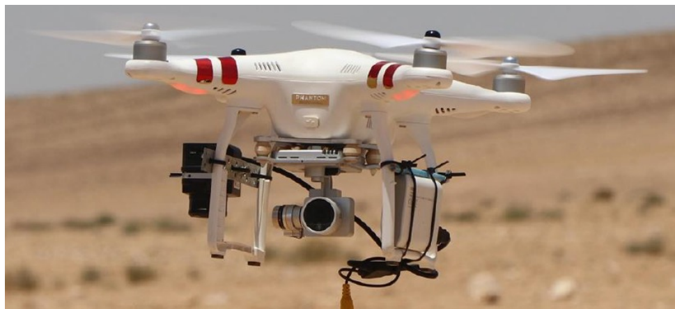
Chart 15: Electro-optical system on a UAV for mine and ERW detection
